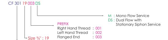
Shaft/Roller that turns anticlockwise: Rotor Thread "RH" Shaft/Roller that turns clockwise: Rotor Thread "LH"
